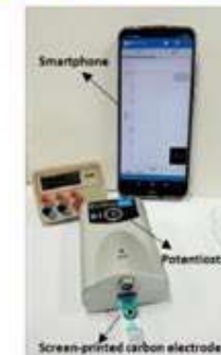
Fig. 1. (Left) Detail of the screen-printed carbon electrode (SPCE) used as sensing platform and transducer; (Right) Picture of the set-up used for the electrochemical measurements.
